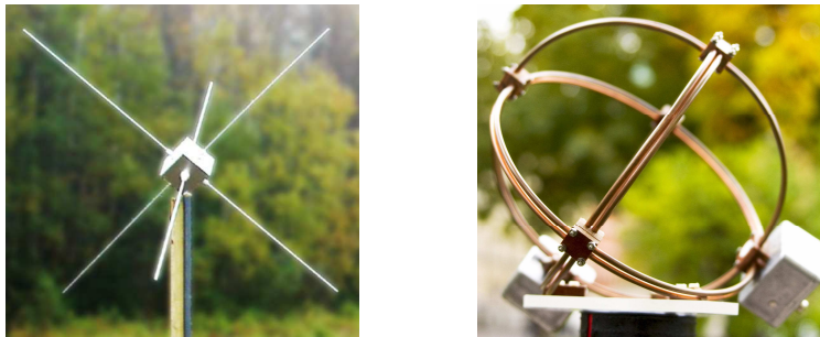
Figure 3.1: LOIS electric and magnetic tripole antennas
